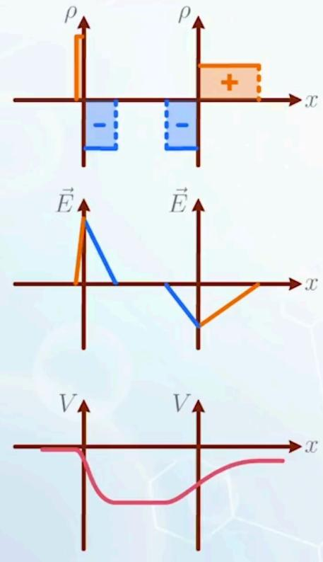
The emitter is usually the most heavily doped region, while the collector is the most lightly doped region.
