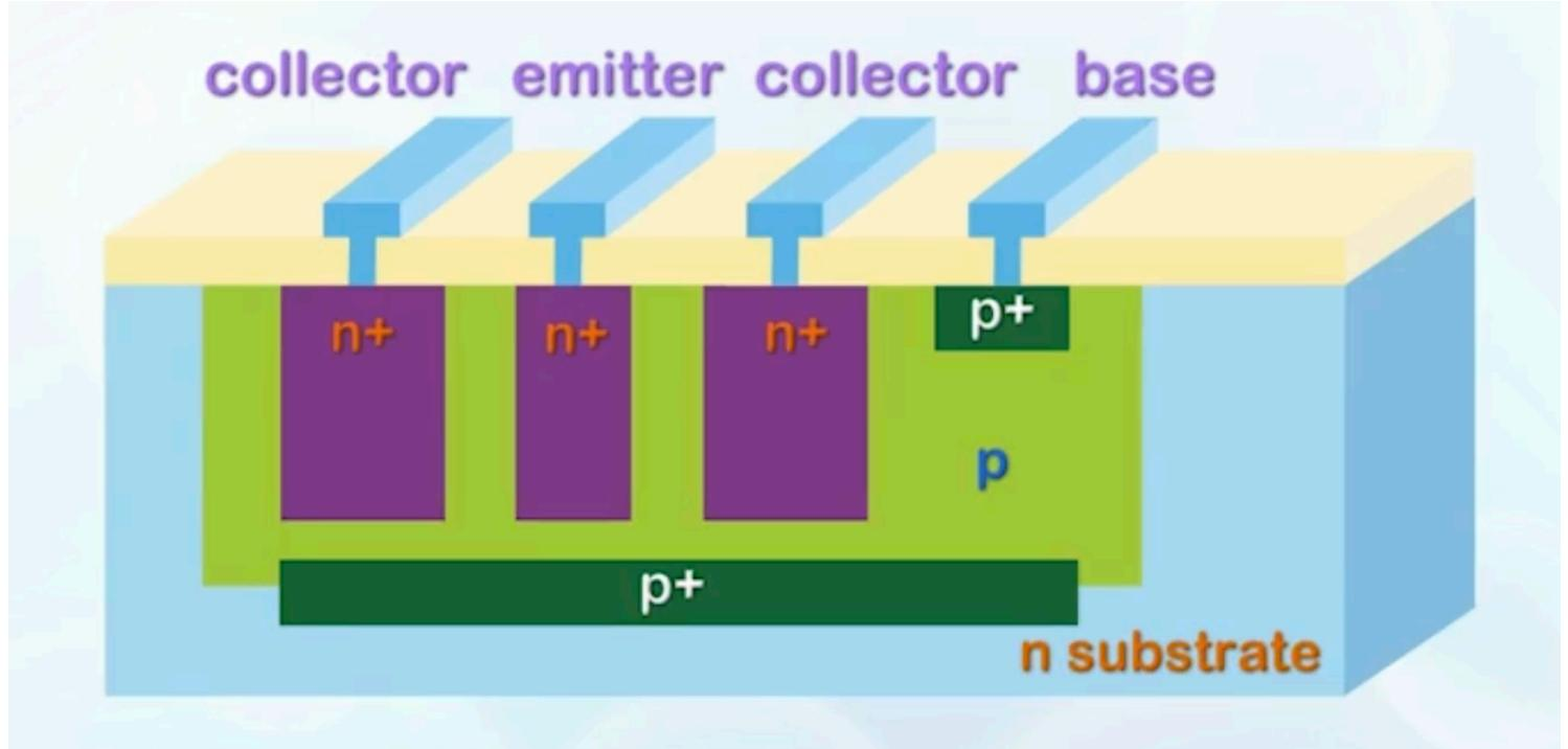
The vertical dimension can be more precisely controlled relative to the lateral dimension in IC processing, the BJT technology is still dominated by vertical BJTs.
