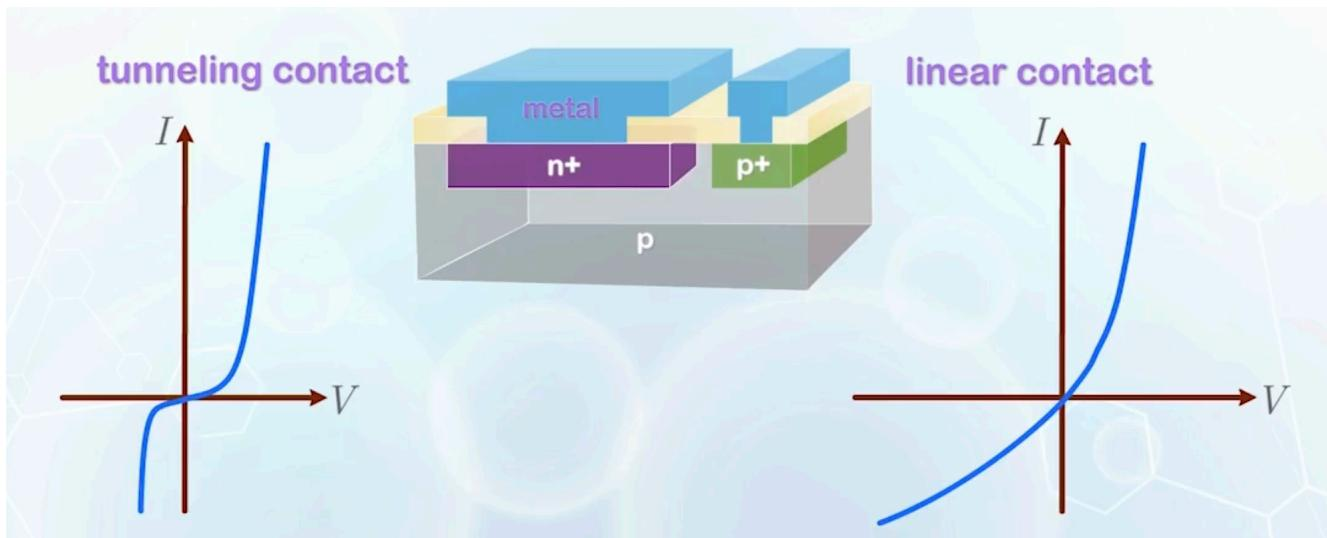
The internal built-in potential of a PN junction will be balanced out by the band bending at the metal-semiconductor contacts, thus the built-in potential cannot be measured.
