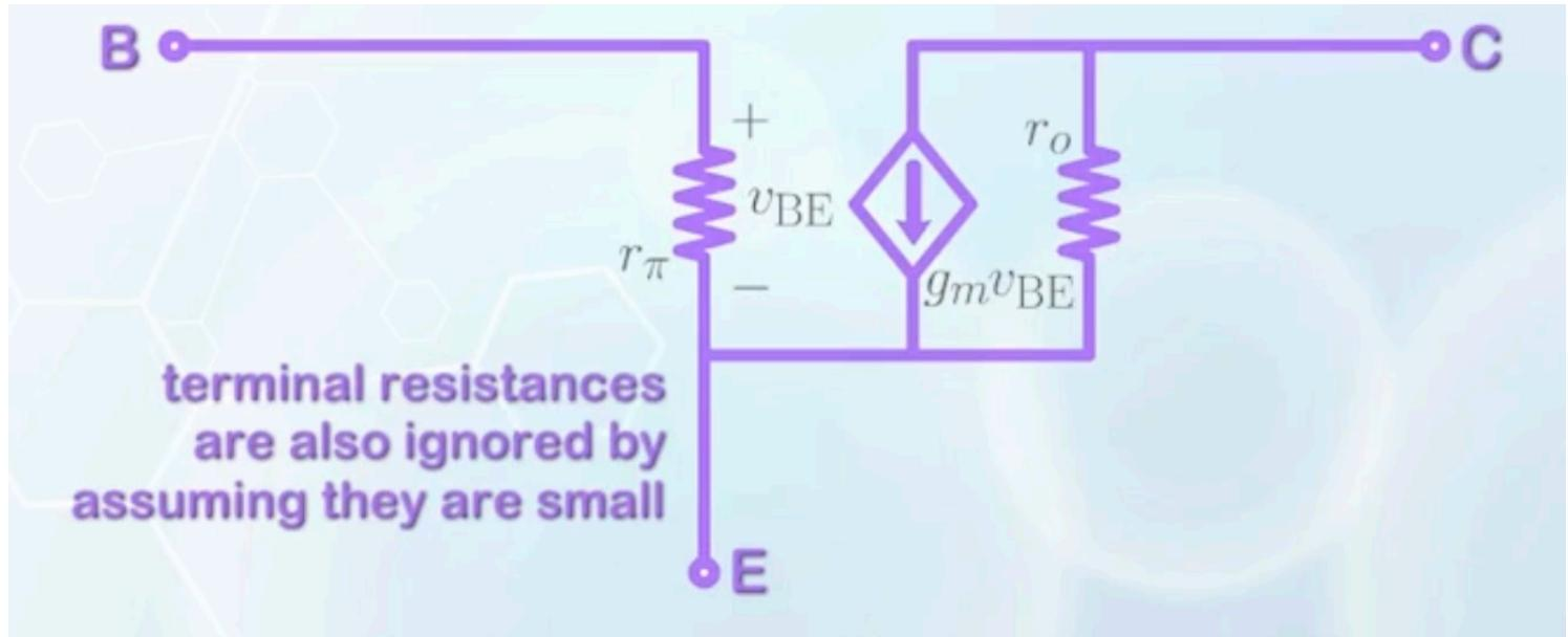
When frequency increases, it is possible that before a carrier can reach the collector, the signal has already been reversed. In such case, the collector current does not respond to the change of the input
